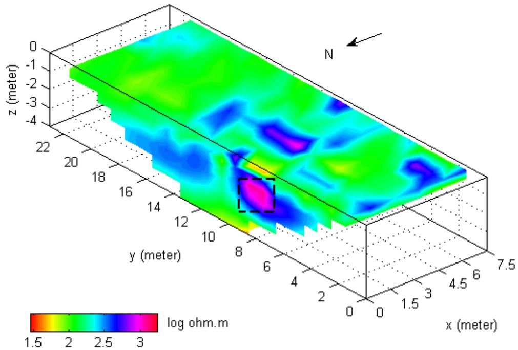
**FIG. 5.** Pseudo three-dimensional geo-electrical model of the investigation area. The high resistivity anomaly (black rectangle) is related to a man-made structure.
