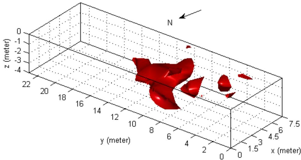
**FIG. 7.** Iso-resistivity surface of the highest resistivity zones ( $> 2.7 \log \text{ ohm.m}$ ).
