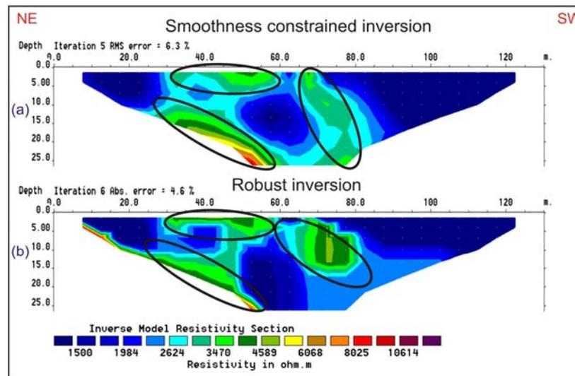
**FIG. 7.** Geoelectric section for line 4 using the smoothness constrained (a) and the robust (b) inversion
