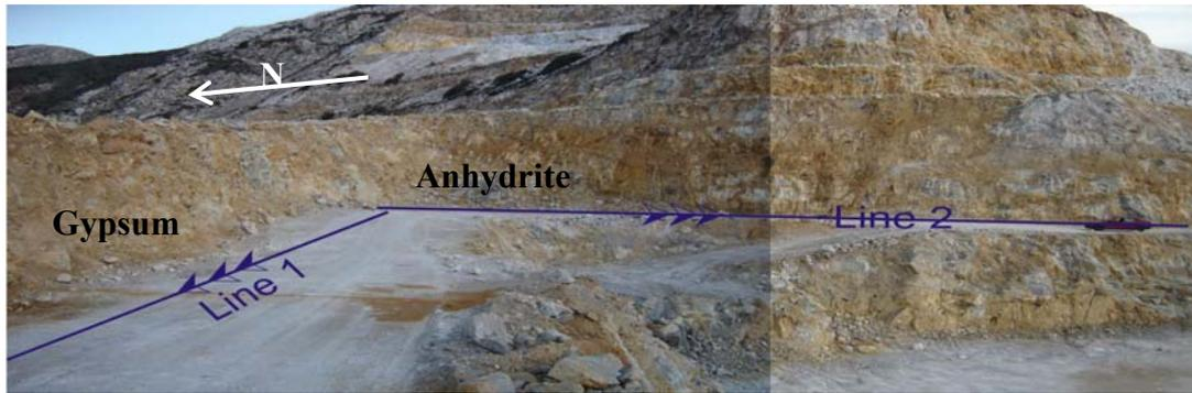
**FIG. 3.** A picture of the bench where ERT lines 1 & 2 took place.
