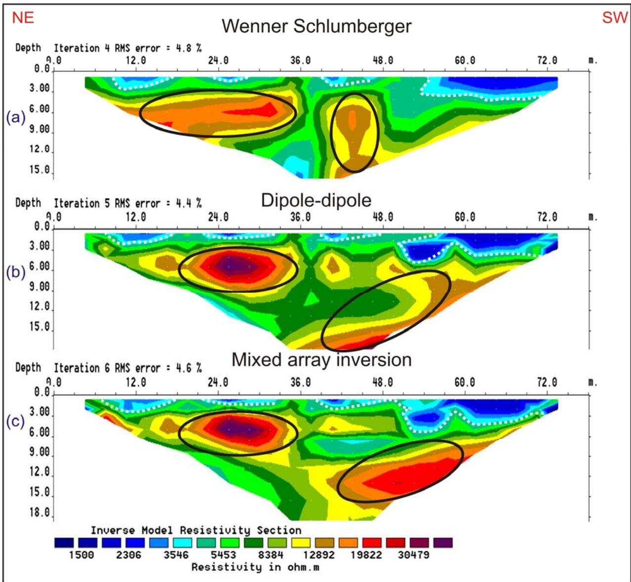
**FIG. 5.** Geoelectric sections for Wenner-Schlumberger array (a), Dipole-dipole array (b) and mixed array (c) of line 2. The black ellipse depicts the anhydrite bodies.
