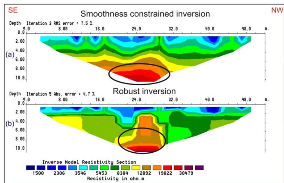
**Fig. 9.** Geoelectric section for line 5 using the smoothness constrained (a) and the robust (b) inversion.
