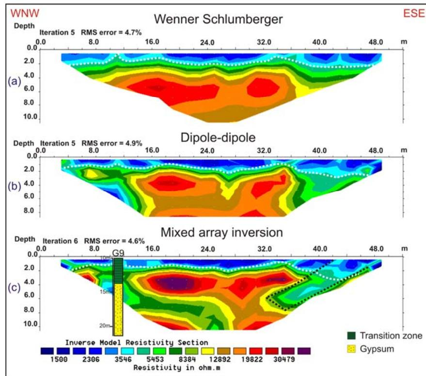
**FIG. 4.** Geoelectric sections for Wenner-Schlumberger array (a), Dipole-dipole array (b) and mixed array inversion (c) of line 1. The dotted black line depicts a gypsum wedge lying underneath the anhydrite mass.
